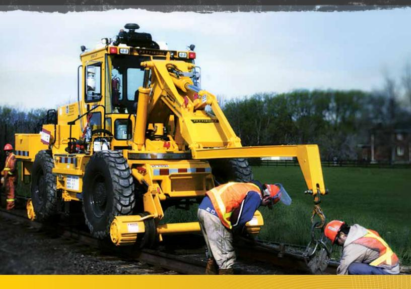
Designed to tackle a variety of rail applications, the Pettibone® Speed Swing™ 445E is a versatile machine that provides the power to lay rails, set ties or clear the path ahead. The unit features a turbo diesel engine and 180-degree boom rotation for enhanced productivity. Offering precise hydraulics, numerous attachments and the ability to work both on and off the rails, the Speed Swing 445E is equipped for any rail task.
